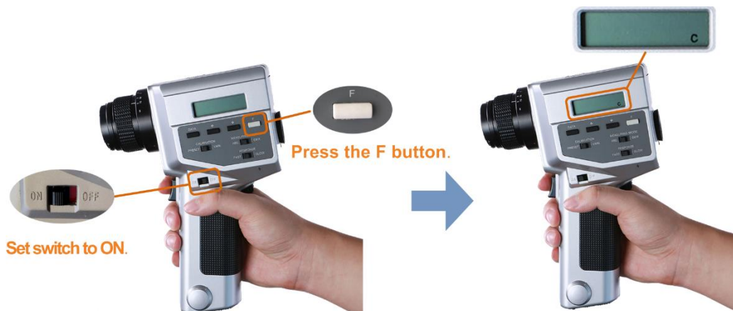
Figure 12-10 Setting CS-100A colorimeter
