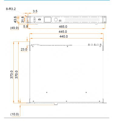
Tolerance: ±0.3 Unit: mm
